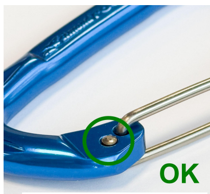
Riveting OK, rounded end in a "mushroom" shape
