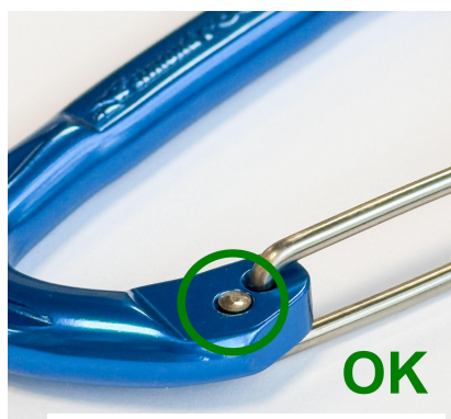
Riveting OK, rounded end in a "mushroom" shape
