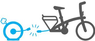
In case of a puncture to the rear wheel, remember to disconnect the motor cable before removing the wheel from the bike to carry out the repair.
